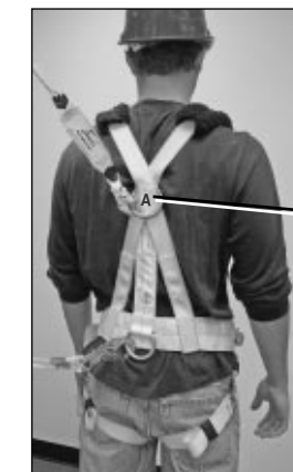
FW-1 in use. "A" marking denotes the point for attachment for tailrope and is stamped in indelible red ink in the center of the dorsal D-ring.
